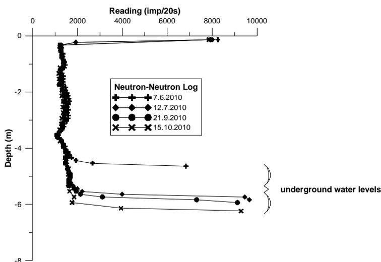
Fig. 1. Results of neutron-neutron logging in the central well.
