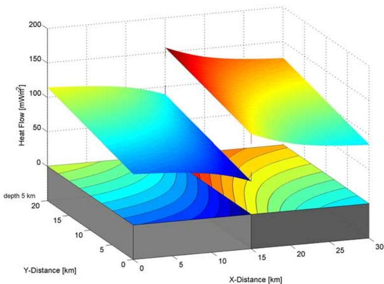
Fig. 1. The distribution of the surface heat flow density over the vertical contact zone with thermal conductivity contrast and with additional heat flow density gradient along the surface boundary of rock blocks. The figure demonstrates the step change in terrestrial heat flow density distribution typical for such contact zones ( and in slightly changed forms also for various model configurations with aslant contacts of blocks).
