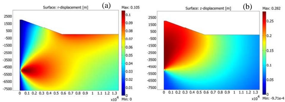
Fig. 1. The computed horizontal (a) and vertical (b) component of the displacement field.
